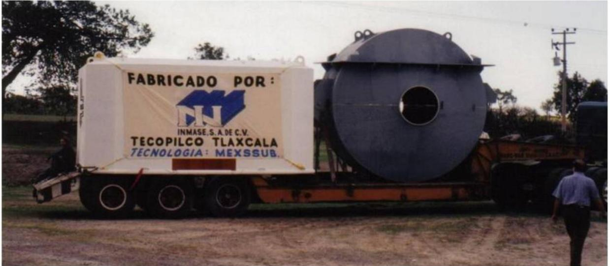
**Manufacture of staple to protect a valve which is 34 m. below sea level. Technology of customer MEXSSUB S.A. de C.V. Sleeve with elbow form & riser for marine platform.**
